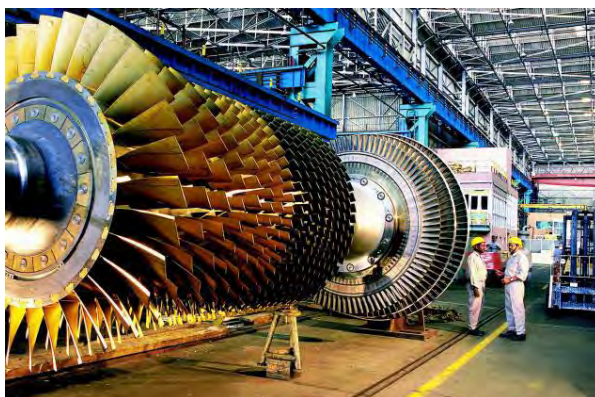
A steam turbine with the outer case removed.
